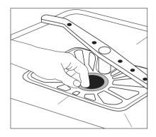
ensure that the flat filter does not protrude above the base of the washing compartment.
